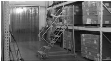
The primary material used for rolling warehouse ladders is steel. Never use steel ladders near electrical hazards due to steel's conductivity. Accidents could result in electrocution. Fiberglass non-conductive rolling ladders are now available and should be used if your work is near electric hazards.
